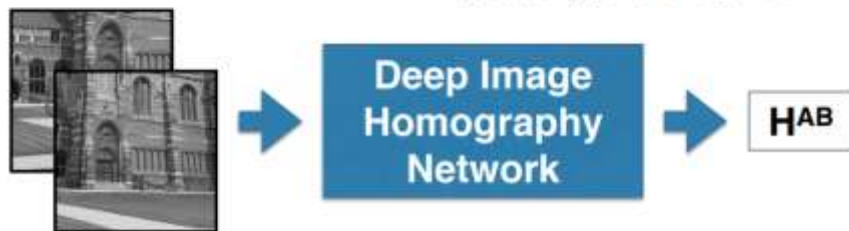
Step 5: Stack Patch A and Patch B channel-wise and feed into the network. Set H^{AB} as the target vector.
